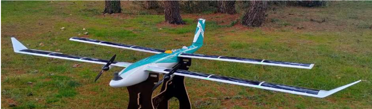
Figure 3 : Xsun's Solar-Powered Long Endurance Surveillance Drone
